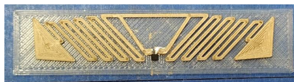
Fig. 4 Fully 3D printed UHF RFID tag made of PLA (substrate) and Electrifi (antenna).
