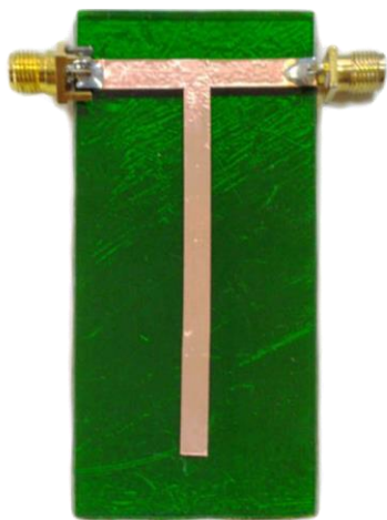
Fig. 12 Resin-made T-Resonator printed with a DLP 3D printer.
