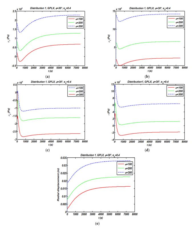
**Figure 8.** Influence of the circular velocity on the transient stress state (**a**–**d**) and radial displacement (**e**) for a center point of truncated cone (D1-GPL X;  $e_0 = 0.4$ ;  $\phi = 30^\circ$ ;  $\gamma_{GPL} = 0.01$ ).
