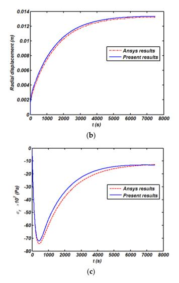
**Figure 2.** Time history of temperature (**a**), radial displacement (**b**), and radial stress (**c**) for a center point of cone compared with ANSYS Workbench.
