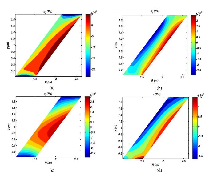
**Figure 12.** Contour of steady stress state (**a**–**d**) (D2-GPL V;  $\phi = 30^\circ$ ;  $\gamma_{GPL} = 0.01$ ;  $\omega = 100 \text{ rad/s}$ ).
