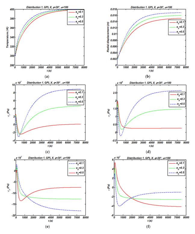
**Figure 6.** Influence of porosity coefficient on the transient temperature (**a**), radial displacement (**b**), and stress state (**c**–**f**) for a center point of truncated cone (D1-GPL X;  $\phi = 30^{\circ}$ ;  $\gamma_{GPL} = 0.01$ ;  $\omega = 100 \text{ rad/s}$ ).
