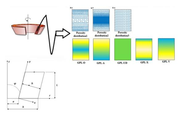
**Figure 1.** Geometry of rotating truncated cone for various porosity and GPL patterns across the x axis (thickness direction).
