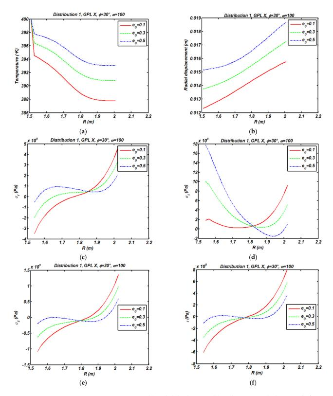
**Figure 11.** Temperature (**a**), radial displacement (**b**), and stress state (**c**–**f**) at z = L/2 for various porosity coefficient (D1-GPL X;  $\phi = 30^\circ$ ;  $\gamma_{GPL} = 0.01$ ;  $\omega = 100$  rad/s).
