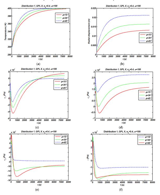
**Figure 5.** Influence of semi-vertex angle on the transient temperature (**a**), radial displacement (**b**), and stress state (**c**–**f**) for a center point of truncated cone (D1-GPL X;  $e_0 = 0.4$ ;  $\gamma_{GPL} = 0.01$ ;  $\omega = 100 \text{ rad/s}$ ).
