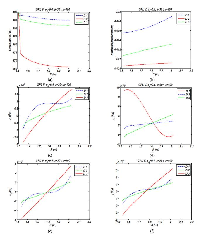
**Figure 10.** Temperature (**a**), radial displacement (**b**), and stress state (**c**–**f**) at z = L/2 for various porosity distribution. (GPL V;  $e_0 = 0.4$ ;  $\phi = 30^\circ$ ;  $\gamma_{GPL} = 0.01$ ;  $\omega = 100$  rad/s).
