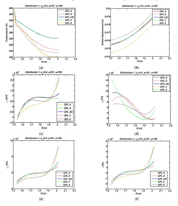
**Figure 9.** Temperature (**a**), radial displacement (**b**), and stress state (**c**–**f**) at z = L/2 for various GPL patterns (D1;  $e_0 = 0.4$ ;  $\gamma_{GPL} = 0.01$ ;  $\omega = 100$  rad/s).
