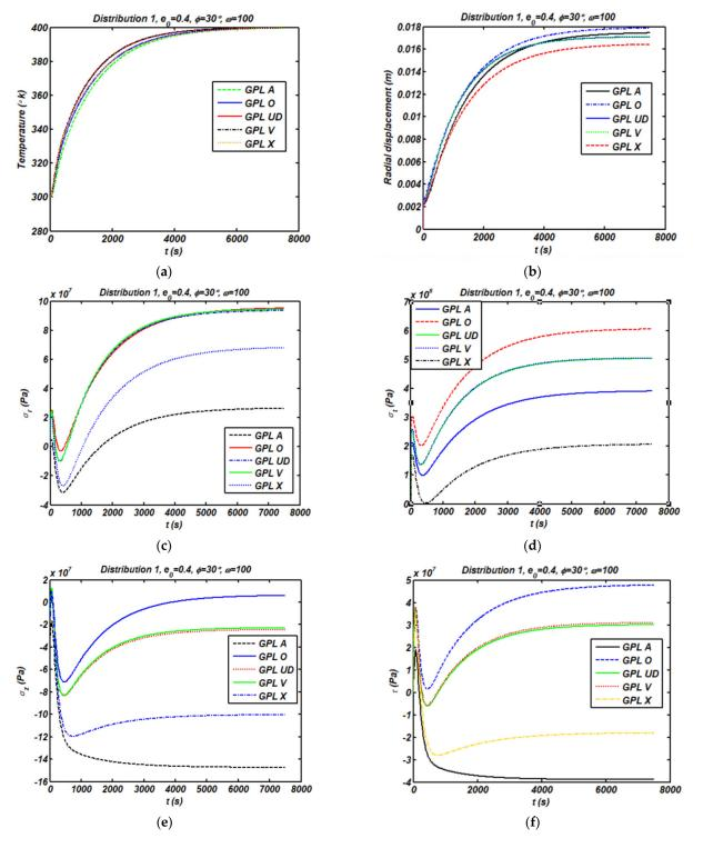
**Figure 3.** Influence of GPL pattern on the transient temperature (**a**), radial displacement (**b**), and stress state (**c**-**f**) for a center point of truncated cone (D1;  $e_0 = 0.4$ ;  $\phi = 30^\circ$ ;  $\gamma_{GPL} = 0.01$ ;  $\omega = 100 \text{ rad/s}$ ).
