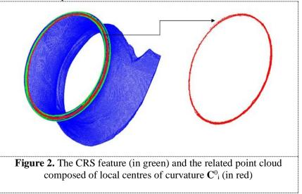
In the following step, a first-attempt sweep line is estimated (it is depicted in green in figure 3). The sweep line consists of a set of n polynomial curves of 2-nd degree  $\gamma_i^0 \equiv (\gamma_{i_x}^0, \gamma_{i_y}^0, \gamma_{i_z}^0)$ . Each of them locally approximates the set of centers of curvature  $\mathbf{C}_i^0$ . The curve segments  $\gamma_i^0$  are evaluated by a moving average filter that locally performs a least-squares robust regression.
