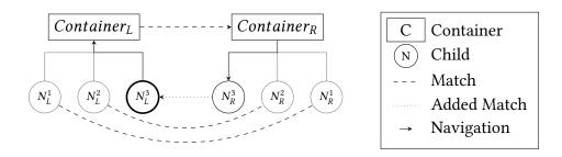
Figure 7.2.: Match Correction for Unmatched Leaves
