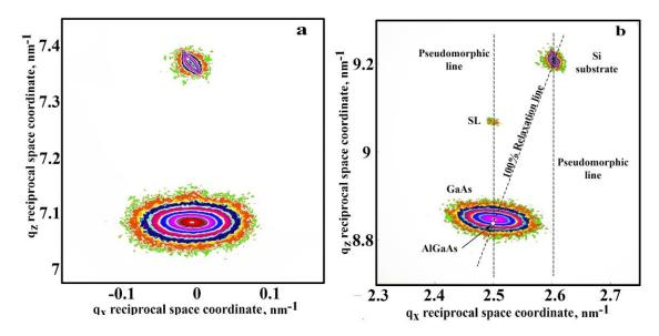
**Figure 2.** XRD mapping images symmetric (004) (**a**) and skew-symmetric (511) (**b**) reflections of GaAs/SL/proto-Si(100) heterostructures.
