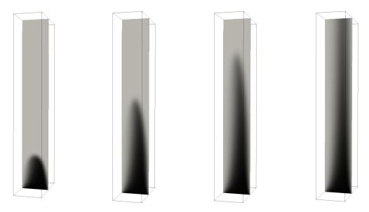
Figure 7.7.: Time evolution of the gas phase in the fluid flow, till steady-state is reached. Black color indicates high  $CO_2$  concentration. The coupling to light supply yields in a consumption of  $CO_2$  close to the left reactor wall.
