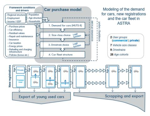
Fig. 1. Overview of the car fleet model in ASTRA.
