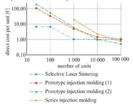
Fig. 4. Costs per unit of different lot sizes and manufacturing processes
