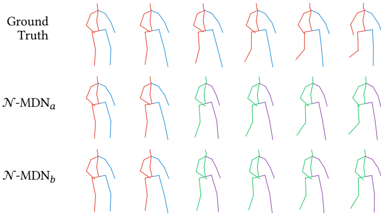
Figure 5.28: Qualitative comparison of predictions generated by both variants of the \mathcal{N} -MDN on the walking action. \mathcal{N} -MDN a generates diagonal covariance matrices. \mathcal{N} -MDN b generates sparse covariance matrices, which model inter-joint correlations. For illustration purposes, the sample rate is reduced to 12.5Hz. For each prediction, the last 2 observed poses are depicted together with an prediction of 320 milliseconds (4 time steps) into the future. The full ground truth sequence of poses is depicted in the first row. The left arm and leg are depicted in blue (ground truth) or purple (prediction), respectively.
