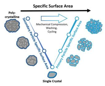
**Figure 11.** Schematic representation of the specific surface areas (SSAs) for different CAM morphologies. The left side represents the secondary, the right side the primary particle SSA that act as boundaries to the minimal/maximal accessible surface area of the CAM. By processes such as mechanical compression, washing and electrochemical cycling, the SSA increases by better accessibilty of the inner pore structure. For single crystal materials, both boundaries converge to a single value.
