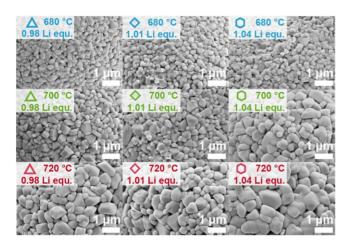
**Figure 2.** Top-view SEM images of the nominal 12  $\mu$ m LNO samples made with different Li equivalents and at different calcinations temperatures (see legends). All images were recorded in 20 k magnification with an acceleration voltage of 5 kV. A 6 nm thick Pt layer was sputtered onto all samples. The length of the white scale bar equals 1  $\mu$ m.
