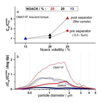
**Fig. 6** a Changes in total mass emission and PSD with volatility relative to the emission at Noack 13% for the OM471P engine in low-end torque operation, measured before and after an oil mist separator. **b** PSDs normalized by the total mass concentration of the OM471P at Noack 25%
