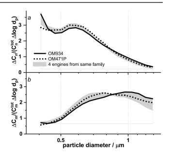
**Fig. 1** Comparison of crankcase aerosol PSD by number (**a**) and mass (**b**) for several engines, including data for four engines from earlier study [14]. These earlier data are represented in terms of a scatter band.  $\Delta$ logdp represents the logarithmic width of particle size classes used by the OPC
