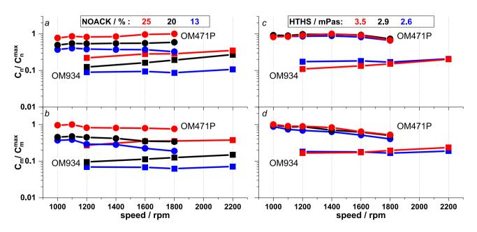
Fig. 5 Impact of volatility and viscosity on total aerosol concentrations by number  $(\mathbf{a}, \mathbf{c})$  and mass  $(\mathbf{b}, \mathbf{d})$  as a function of engine speed at full load. All concentrations are relative the maximum total concentration of the OM471P
