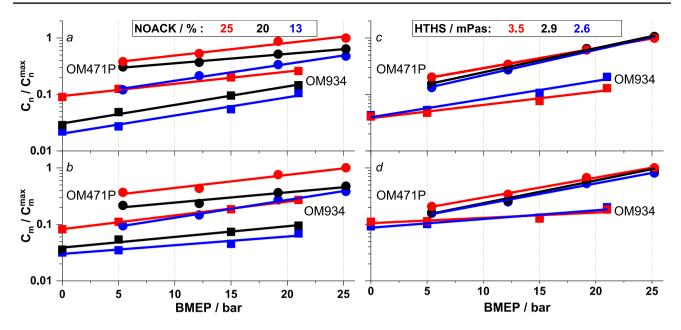
**Fig. 4** Impact of volatility and viscosity on total aerosol concentration by number  $(\mathbf{a}, \mathbf{c})$  and mass  $(\mathbf{b}, \mathbf{d})$  as a function of engine load (expressed as BMEP) at a fixed engine speed of 1100 and 1200 rpm,
