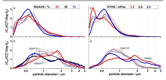
Fig. 3 Impact of oil volatility and viscosity on aerosol particle size distributions based on number (a, c) and mass (b, d) concentration. Measurements are at the low-end torque engine operation point. PSD
