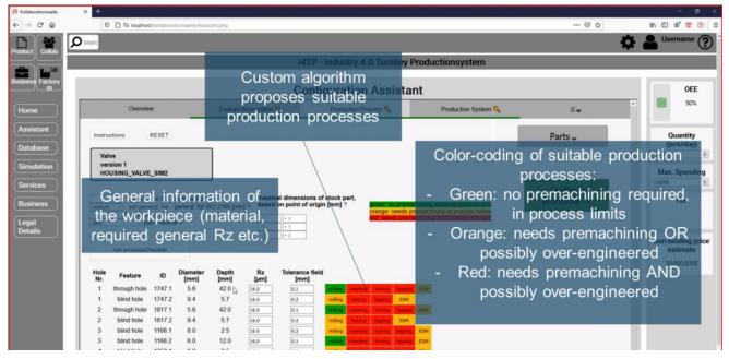
Figure 10 Proposition of suitable production processes based on the identified features
