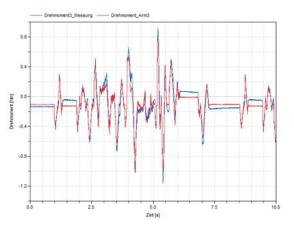
Figure 26 Measured and simulated torque
