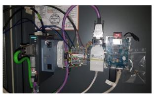
Figure 34 Use of the Smart Controller to integrate a Schaeffler SpindleSense sensor
