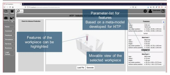
Figure 9 Feature Extractor application on the I4TP platform
