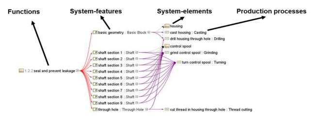
Figure 4 Traceability between different elements in a SysML model
