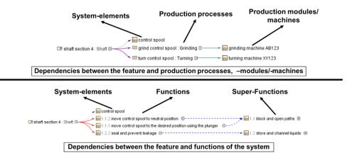
Figure 23 Analysis of the direct and implied dependencies from the feature shaft section 4
