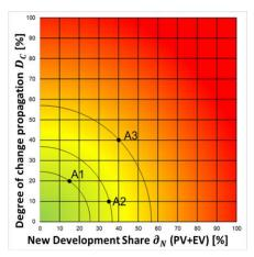
Figure 22 Diagram for the visualization and comparison of the calculated risk  $R_D$  for different design decisions/engineering changes (adapted from Albers et al. 2021)
