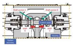
Figure 21 Section through the hydraulic valve, exemplarily displaying the parts "control spool" and "housing" as well as the features "shaft section 4/6" of the control spool
