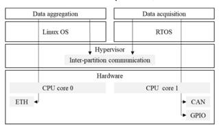
Figure 39 Smart Controller Architecture
