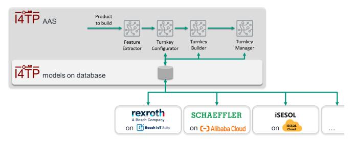
Figure 2 Architecture of the I4TP platform
