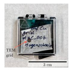
Figure 5.6. Storage box for aC films on TEM grids that serve as contamination test specimens.
