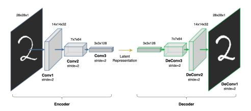
Figure 2.5: Example of a convolutional autoencoder. Adapted from [34].
