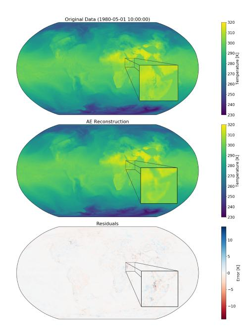
Figure 5.9: Reconstruction of the original data with the convolutional AE.
