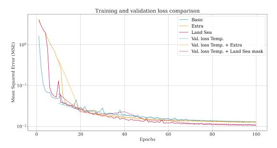
Figure 5.5: Train and validation losses achieved by the models with different inputs.
