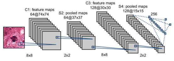
Figure 2.3: Example of a CNN architecture [29].
