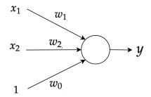
Figure 2.1: Perceptron with two inputs and one output.
