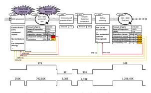
Fig. 8. Quality Value Stream Visualization of target state
