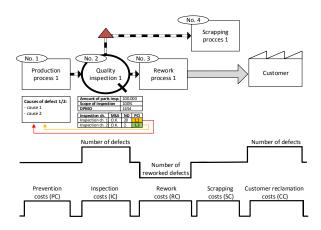
Fig. 4. Illustration of a value stream including defect and quality cost curve
