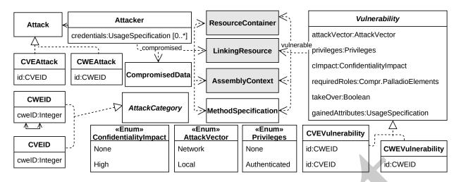
Fig. 3. Simplified metamodel for attackers and system vulnerabilities
