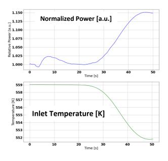
**CAREM Cold Water Transient: Power and** core inlet temperature evolution
