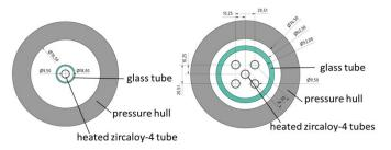
Cross-sectional view of the two planned test arrangements
