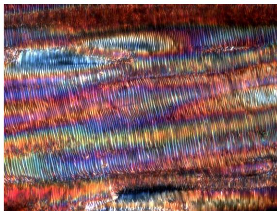
**FIGURE 4** Optical microscope photograph for P20-Cu: shear bands induced on the melt polymers and preserved at room temperature.
