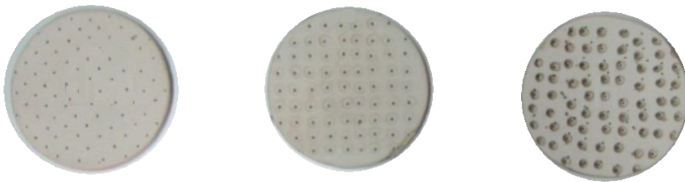
Figure 1. Specimens in ceramic material, with different thicknesses and percentages of perforation.
