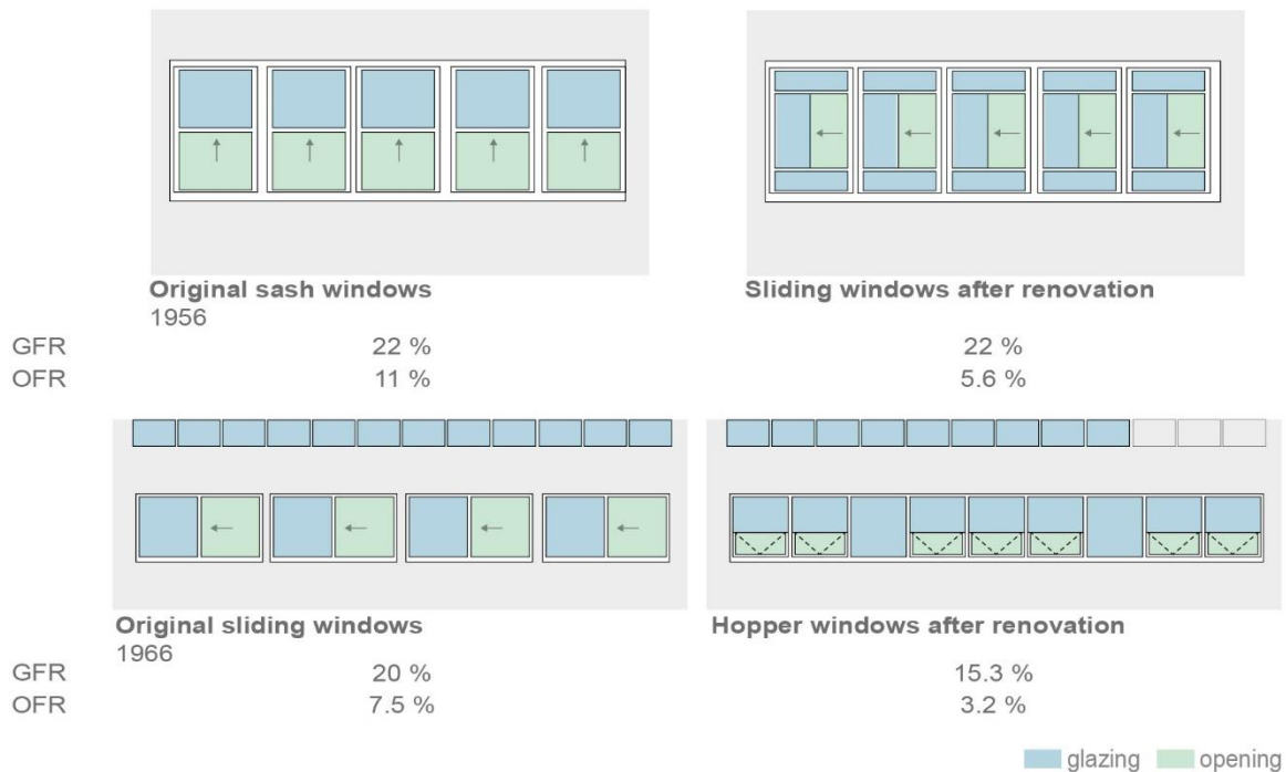
Figure 13. Transformation of window opening type and reduction of opening area in two schools, from original construction to renovation (GFR: glazing to floor area ratio, OFR: opening to floor area ratio).
