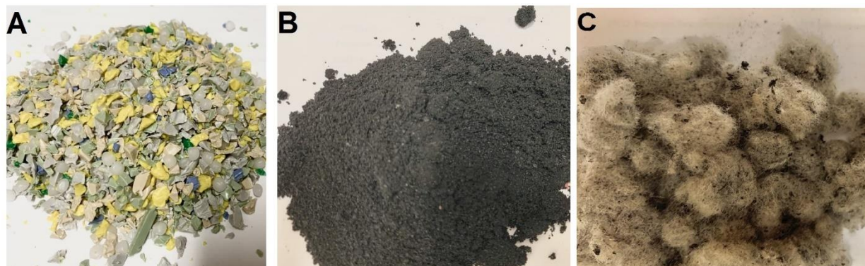
Figure 6.1 General view of the (A) rHDPE flakes, (B) RR particles and (C) RTF as received.
