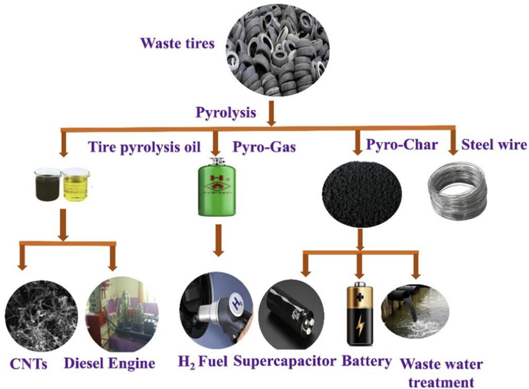
Figure 2.3 Waste tire pyrolysis products and their applications. Adapted from reference [136].
