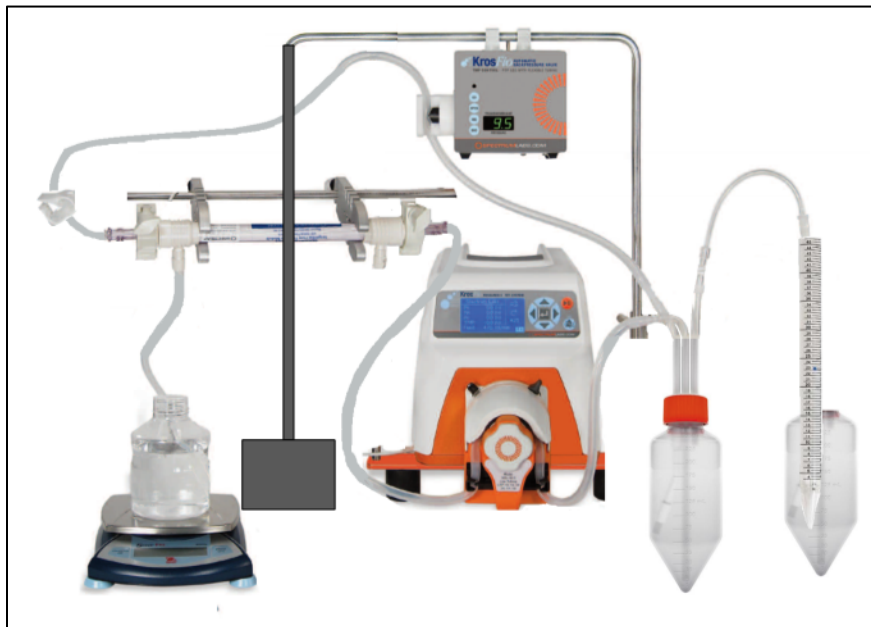
Fig 7. Tangential flow ultrafiltration setup, including the peristaltic pump, feed, pressure gauge, and the TFF cartridge.
