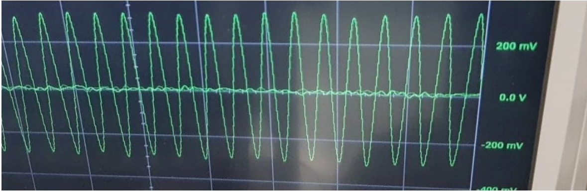
Figure 3.6: Enlarged bursts from the ZigBee device TI 1 with amplitude higher than 40 mV.
