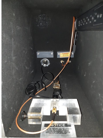
Figure 3.3: Device and antenna in the shielded box (anechoic chamber).
