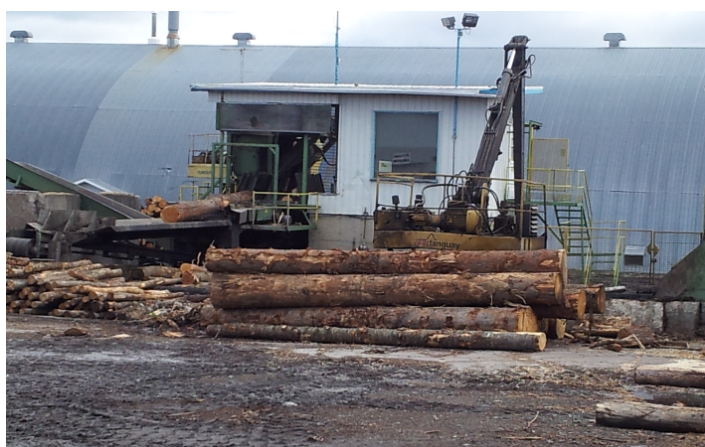
FIGURE 1.4 – Station fixe de tronçonnage.
