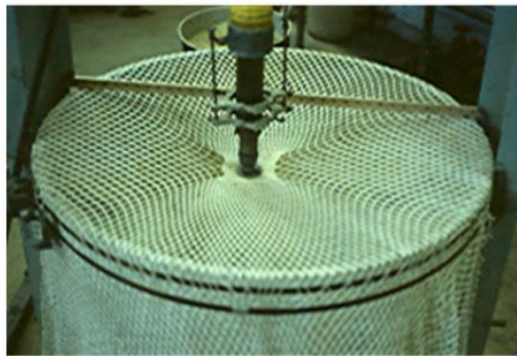
Fig. 2.29. Laboratory testing of specially designed knit geotextile (Koerner, 2015).
