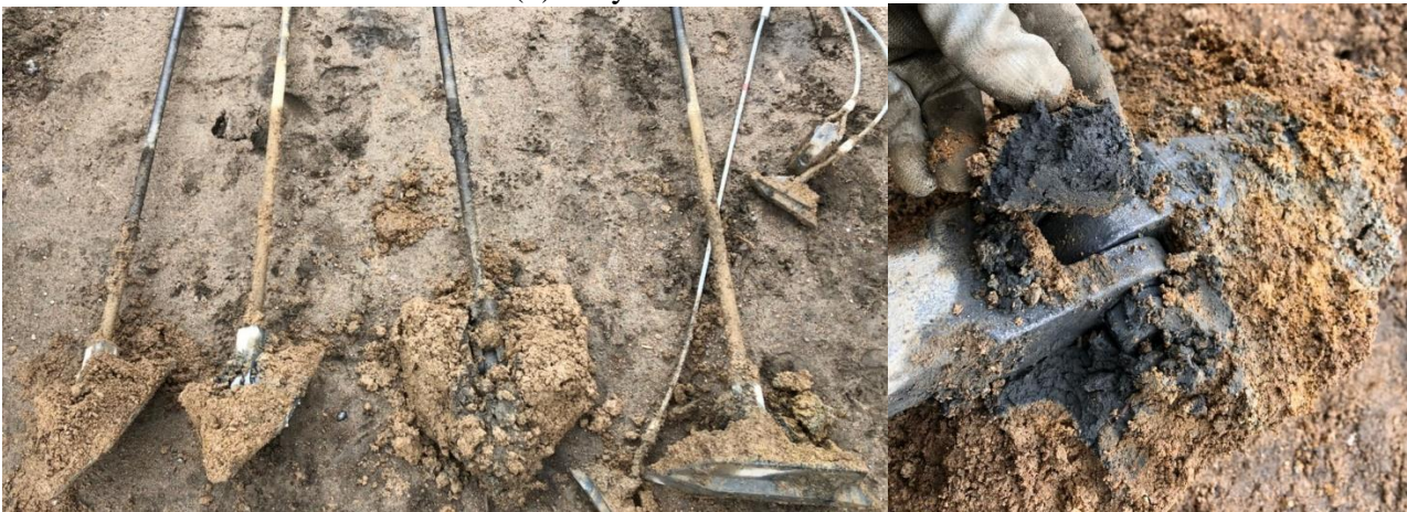
(c) Clay left on anchor heads.
