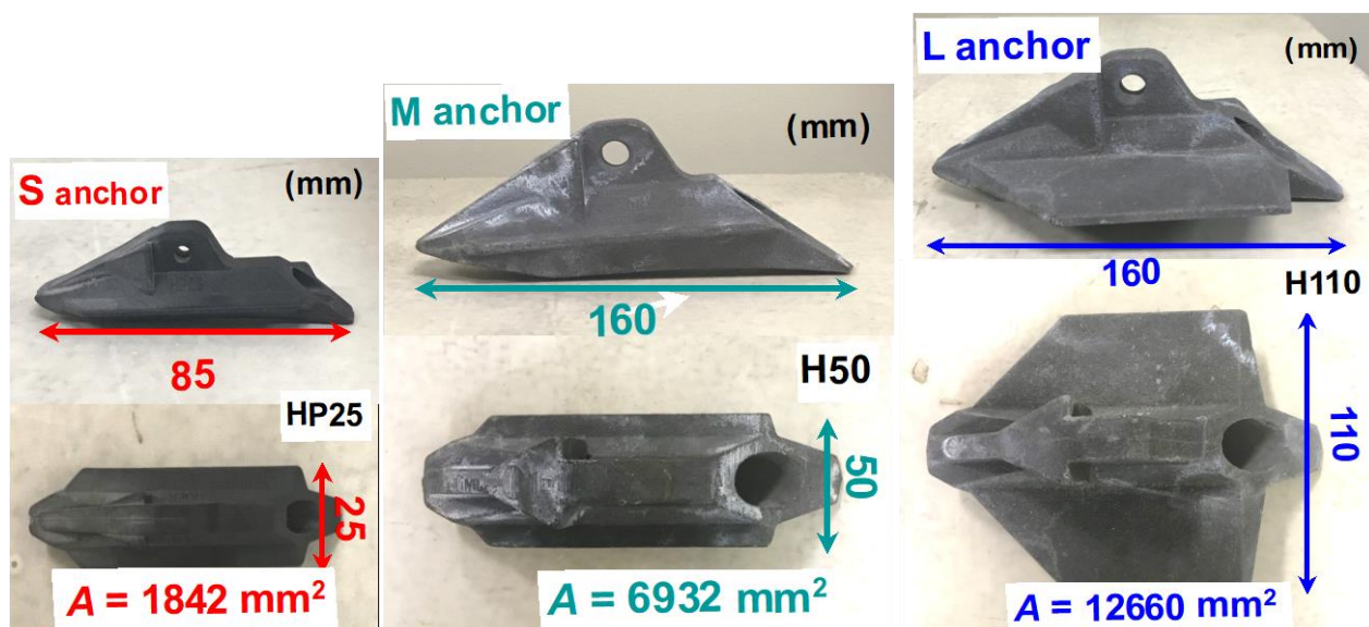
Fig. 3.3. Actual flip anchors (S, M, L) used for pull-out experiments in a laboratory.
