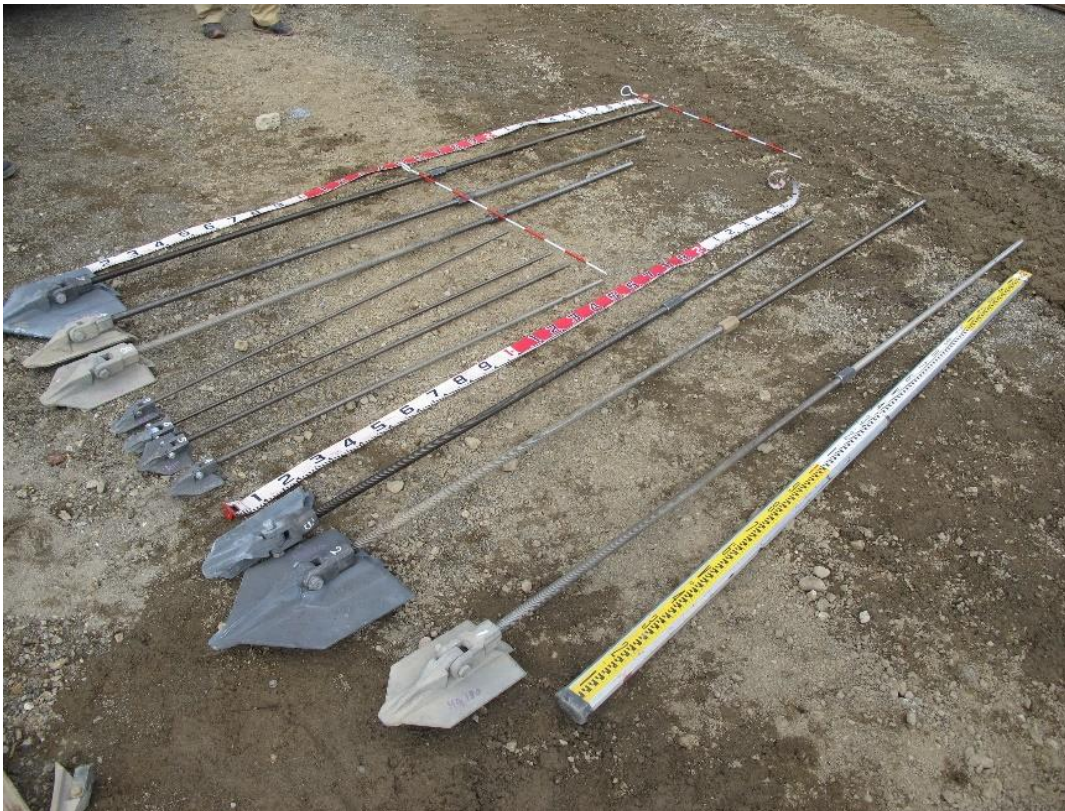
Fig. 3.34. Actual flip anchors used for full-scale pull-out experiments in a field.
