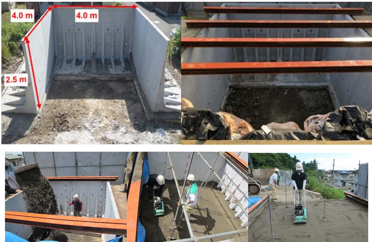
Fig. 3.28. A model ground for pull-out experiments of actual flip anchors in a field.
