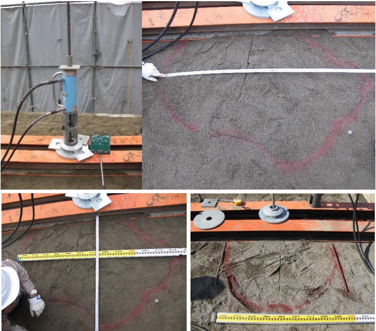
Fig. 3.52. Influenced area of the ground surface by pulling out an anchor (HG320 H = 1.3 m).
