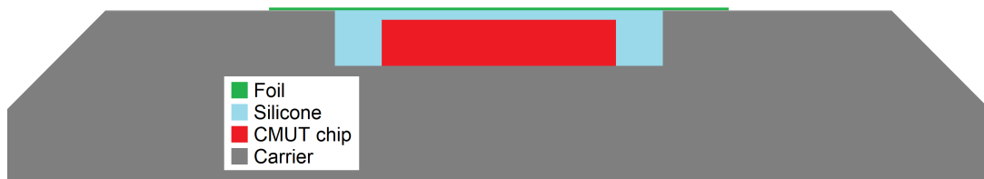
Figure 4.19: Schematic drawing of the experimental encapsulation setup.
