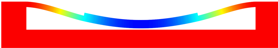
Figure 2.5: Schematic: Bending of a CMUT membrane.
