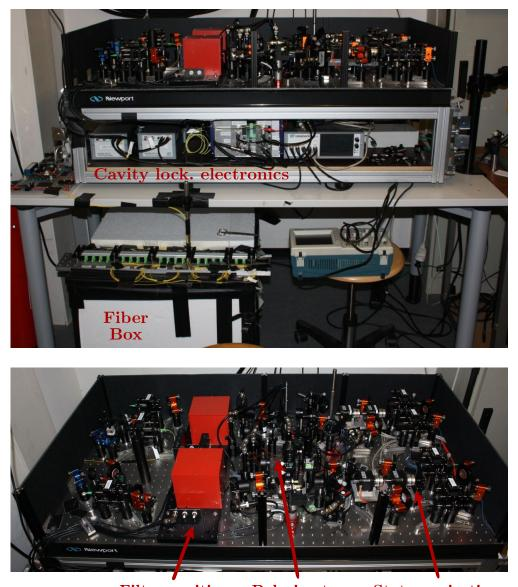
Filter cavitiesPolarimeterState projectionFigure D.3. Platform containing the BSM and spectral filtering system.
