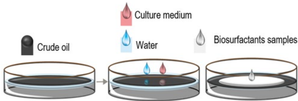
Fig. 4 The oil spread test occurs with the addition of water and a smaller volume of oil to form a thin hydrophobic layer. Then, the test sample is added over the oil layer and provides the displacement of the area on the oil surface
