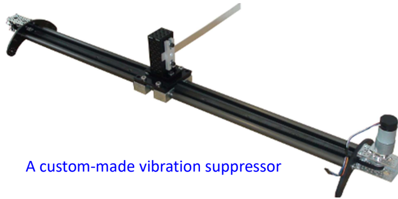
Figure 6.2: A custom-made vibration suppressor developed in the CDR Lab, Control Systems Centre, University of Manchester, for testing the NI controller synthesis algorithms.
