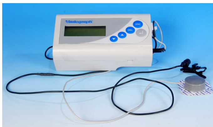
Figure 2.1 VitaloJAK cough monitor showing the device, air microphone and adhesive chest sensor
