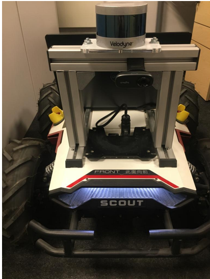
Fig. 5. The Scout 2.0 mobile robot platform provided with modified hardware architecture
