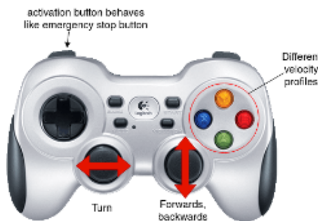
Fig. 6. Joystick key-specific functions applied to our system.
