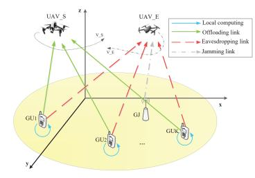
Fig. 1. The NOMA-based UAV-MEC system with a flying eavesdropper.
