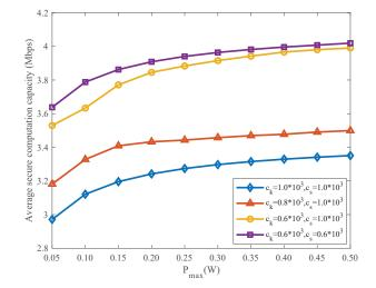
Fig. 8. Average security computation capacity variation with different  $c_s$  and  $c_k$ .
