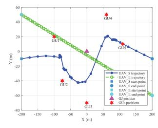
(b) UAV\_S and UAV\_E trajectory with  $P_{max} = 0.1W$ , T = 30s.
