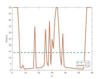
(b) UAV\_S and UAV\_E flight speed with  $P_{max} = 0.1W$ , T = 30s.
