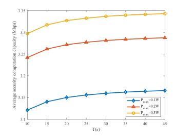
Fig. 7. Average security computation capacity variation versus T with different  ${\cal P}_{max}.$
