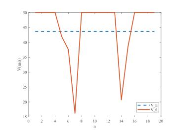
(a) UAV\_S and UAV\_E flight speed with P<sub>max</sub> = 0.1W, T = 10s.
