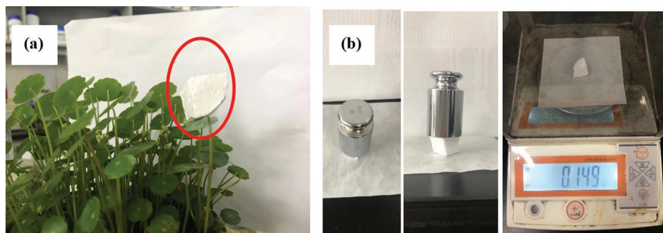
Figure 12. Demonstration of physical properties of the foam (lightness and strength): a) as-prepared foam placed on plant leaves, and b) the foam material withstanding a standard cylindrical weight of around 1340 times its own weight.
