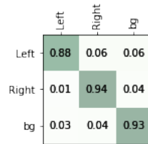
Figure 6.15: Handedness Confusion Matrix on the test set using the final multi-label FR-CNN model
