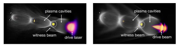
**Fig. 4.9:** Simulation of a LWFA (*left*) and a PWFA (*right*), showing the formation of the accelerating cavities in the plasma. The witness beam is located at the point where the accelerating field is highest, just before the end of the first bubble.
