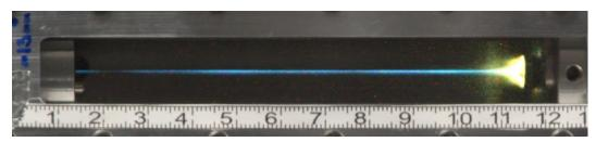
**Fig. 4.8:** Photograph of the visible plasma emission from a 100 mm long hydrodynamic optically-fieldionised (HOFI) plasma channel. The scale visible at the bottom of the image is in cm. Note that the apparent decrease in plasma brightness near a scale reading of 2.5 cm arises from blackening of the cell window in that region, not from non-uniformity of the plasma channel. (*Image credit: A. Picksley, Oxford.*)
