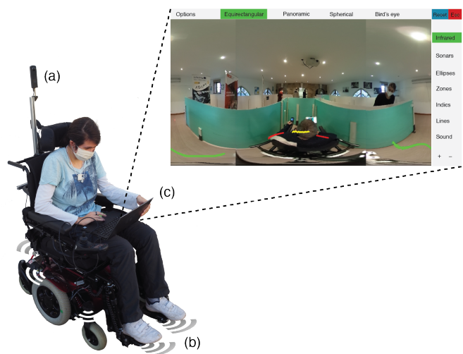
Fig. 6. Basic system components of SpheriCol. (a) Twin-fisheye camera, (b) wheelchair equipped with a ring of ToF sensors, and (c) user interface displaying a panoramic image of the surrounding environment, with coloured distance markers overlaid.
