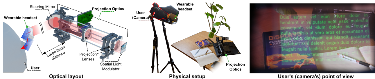
Figure 1. Beaming Displays. Left: Our new optical layout decomposes a near-eye display design into two parts, an all passive light-weight wearable headset, and a remotely located projector, this decomposition effectively avoids trade-offs between ergonomics, computational and power requirements. Middle: We build a physical setup to demonstrate the possibilities with our optical layout. Right: We show experimentally that our design supports resolutions matching a consumer level near-eye display.
