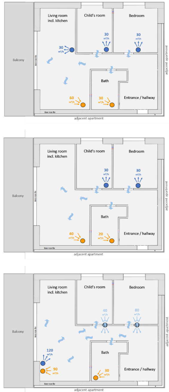
Figure 3-36 Schematic sketch of the simulated ventilation concepts. Top: Reference MVHR, Center: extended cascade ventilation, Bottom: active overflow concept.
