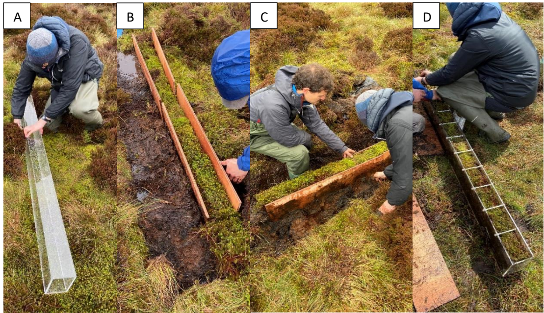
Figure 3.4. Sample extraction methods. A: using the flume tank as a template for extraction; B: plywood planks inserted into grooves alongside sample and removal of material around the sample; C: cutting underneath the sample; D: insertion of sample into flume tank and securing with nylon rods.
