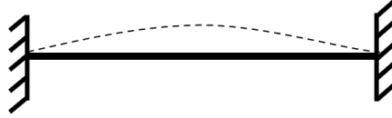
Figure 3.4 Buckling of restrained bar due to the force P.
