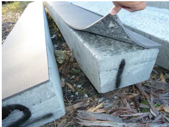
Figure 8.1 USP glued to the sleeper (Kaewunruen et al., 2017).
