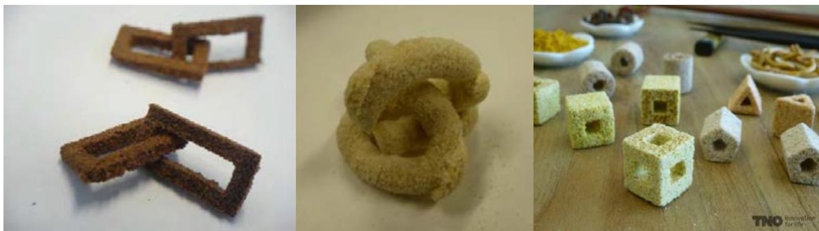
Figure 2-13: Selective laser sintering of food powders. TNO Nesquik powder (left), sugar (middle) and spice powders (right) (van der Linden, 2015).
