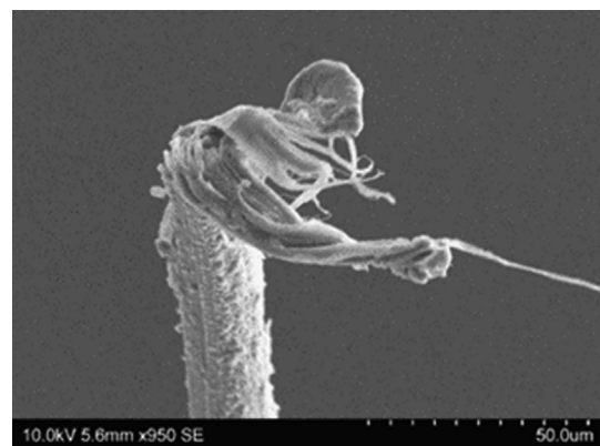
Fig. 7. SEM image of a Dyneema®SK76 filament extracted from a tested yarn.
