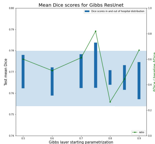
FIGURE 16. Inference of Gibbs-stylized models trained using the Gibbs ResUnet. The upper and lower boundaries of the blue band mark the in- and out-of-distribution mean Dice scores for the baseline model, respectively.
