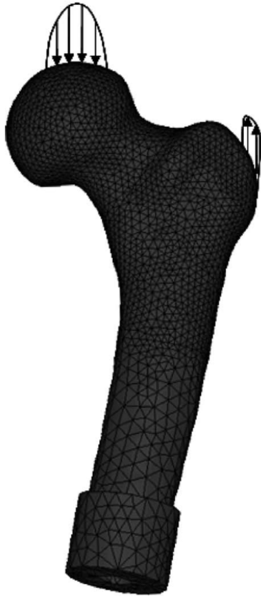
Figure 4.2 The femoral rig fixes Sawbone in 12° of flexion and 12° of adduction.
