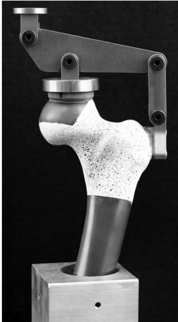
Figure 4.2 The femoral rig fixes Sawbone in 12° of flexion and 12° of adduction.
