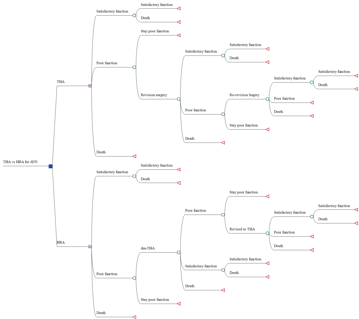
Figure 3.2. This shows how the whole Markov model runs: 3 health states exist after both primary THA and HRA surgery: satisfactory function, poor function and death. Deaths are attributed to the group with satisfactory function. Similarly, 3 health states exist after surgery: satisfactory function, poor function and death. A poorly functioning HRA may be left in situ or revised with a dual-mobility total hip arthroplasty, while a poorly functioning THA may also be left in situ or revised with a revision THA. All these events may result in 3 health states: satisfactory function, poor function and death. Poor function may be treated by revision, or left as a poorly functioning hip. A dual mobility THA may be revised to a revision THA, while a revision THA may be revised to a second revision THA.
