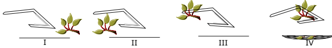
Fig. 3: VRdrone: a leaf-sampling drone in cutting sequence. The bladed mechanism can sample leaves with drone manoeuvres.
