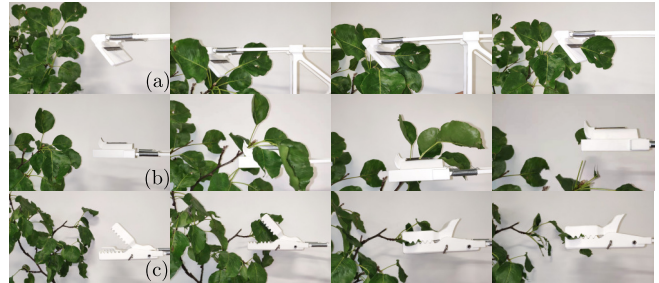
Fig. 5: Leaf sampling sequences from left to right: sampling drone with basket mechanism - (a) comb-like mechanism; (b) vertical blade mechanism; (c) trap-like mechanism activated by the force.
