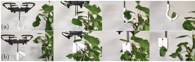
Fig. 7: Small drone for leaf sampling (from left to right) - (a) comb-like mechanism attached from the bottom; (b) passive trap-like mechanism for the sample collection from top.
