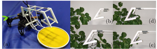
Fig. 4: VRdrone: sampling drone with basket mechanism - (a) a small scale drone endowed with sampling mechanism; (b) the approaching phase; (c) homing the holding branch; (d) taking the leaf into the hook; (e) collecting the leaf phase.
