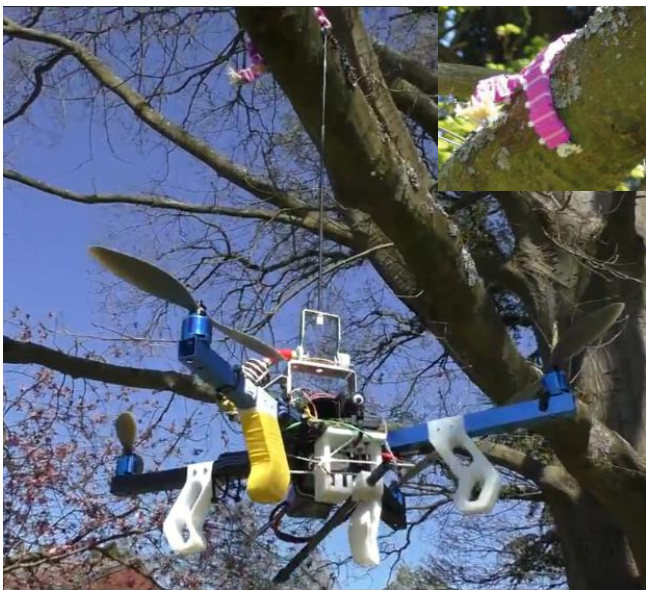
Fig. 8: SpiderMAV: A sequence of images for tensile perching [24]. With the use of microspines that holds the branches, the platform can stay in idle mode.
