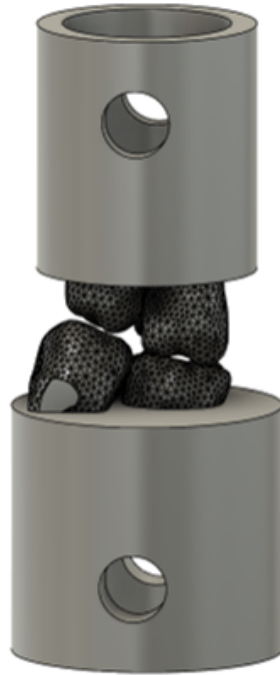
Figure 5.2: The pair of the last two molar teeth was 3D printed as a continuous specimen with adaptors, allowing the proper alignment in the Instron universal machine.
