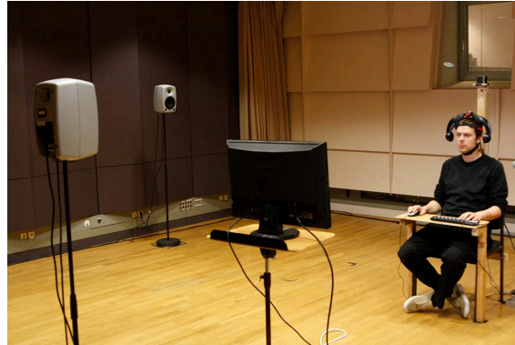
Fig. 5.3 Listening test setup for testing authenticity and plausibility. For seamless switching between audio from the loudspeakers and their binaural simulation, the subject is wearing extraaural headphones that minimize distortions of exterior sound fields. The head position of the subject is tracked by an electro-magnetic sensor pair mounted on the top of the chair and headphones. See also Section 5.4.1.1 (CC-BY, Fabian Brinkmann).
