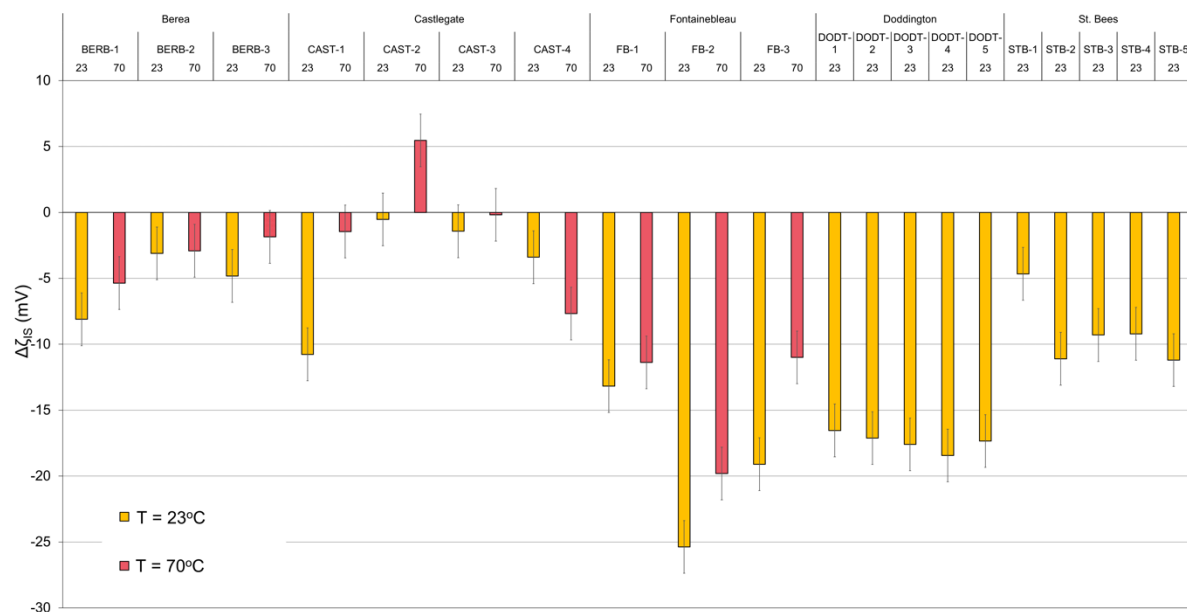
Figure 4-4: Difference between zeta potential measurements obtained on natural, intact sandstone core samples when saturated with high and low ionic strength brines representative of those found in subsurface environments. Yellow bars represent measurements obtained at ambient laboratory temperature (23 °C) and pink bars represent measurements obtained at elevated temperature (70 °C).
