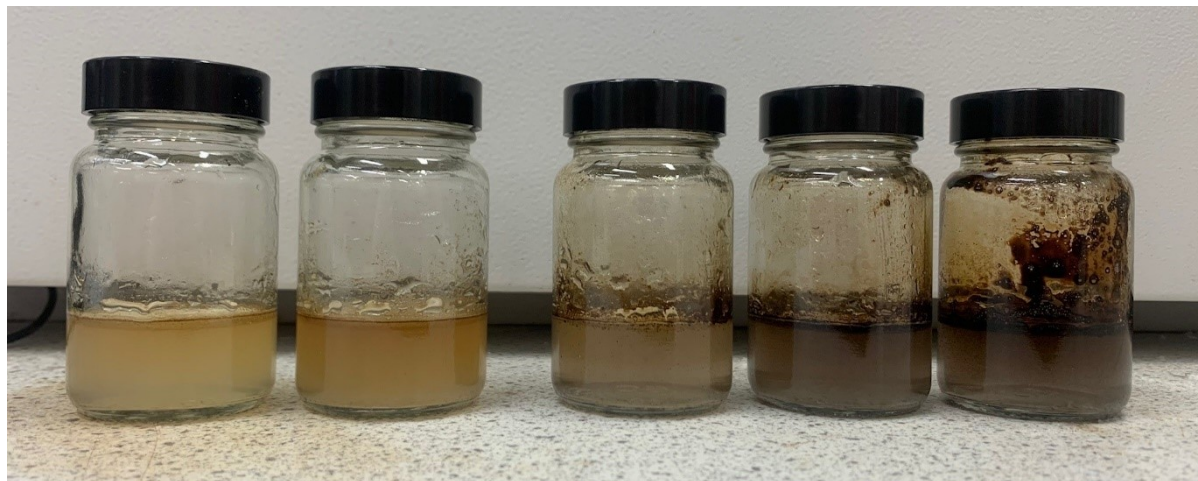
Figure C 1: Emulsions of the five different oils in 0.001M NaCl brine. From far left: Oil T; Oil D; Oil M; Oil P; Oil G.
