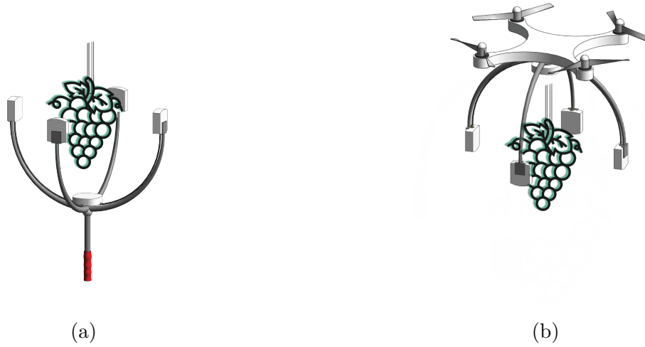
Figure 5.3: (a) Illustration of outdoor SING as a handheld device, and (b) illustration of outdoor SING as an aerial device
