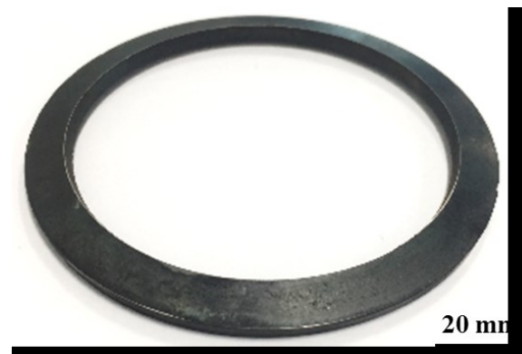
Figure 6.14 Formed disc spring with good surface quality.
