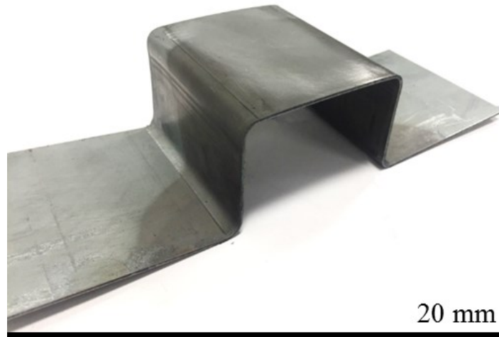
Figure 5.1 Fast-warm stamped demonstrator U-shaped part from MS1180 steel sheet.
